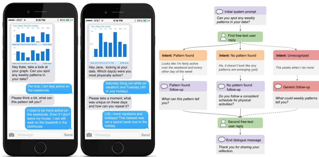
Fig. 1. Example of an actual user exchanges with our system’s mini-dialogues on the left. On the right a block diagram of an example dynamic mini dialogue with: actual user replies, user intents recognized based on free-text replies, and the system tailored follow-ups. The red boxes represent a path where user reply was not recognized and has been handled by a “generic” (non-tailored) follow-up.
